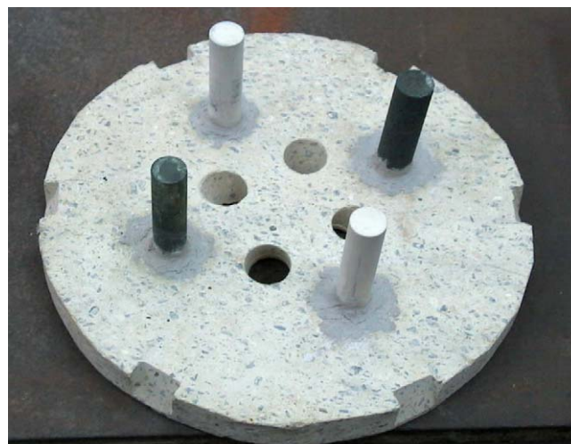
Fig. 2. Mullite plate used as top of the rotary furnace in the specially developed apparatus for the “Merry go Round test” (Fig. 1), before the test. The arrangement of the test specimens (black: cromite, white: electrofused) and the four holes for the burners are observed.
