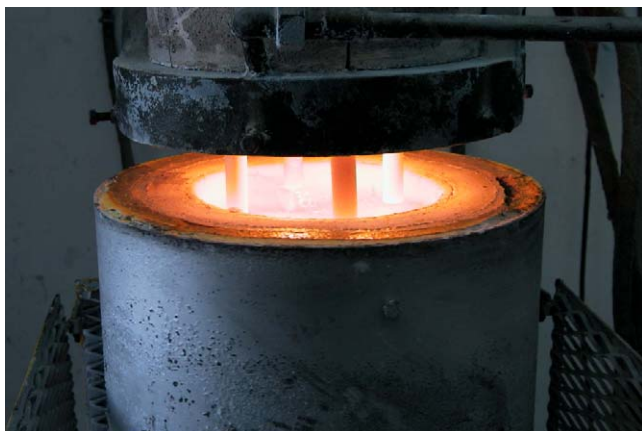
Fig. 1. Specially developed apparatus for the “Merry go Round test”, used in this work. The mullite plate used as top of the rotary furnace is slightly elevated to show the arrangement of the four test specimens. The crucible is filled with the molten frit.
