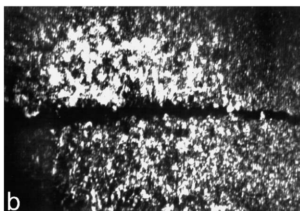
Fig. 5. TEM dark field image pair of twinned corundum produced by dehydration at 600^\circ\text{C} . Images (a) and (b) taken with the reflections used for Fig. 4.
