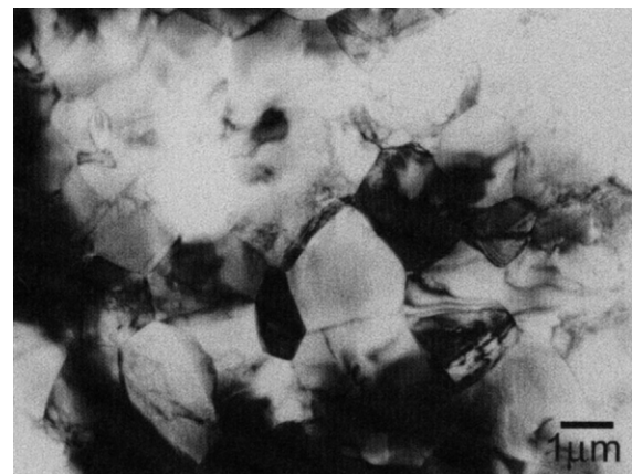
Fig. 3. TEM micrographs of \text{Ba}(\text{Mg}_{1/3}\text{Ta}_{2/3})\text{O}_3 materials incorporated with 0.1 mol% \text{Ba}_5\text{Ta}_4\text{O}_{15} , BaT, showing fine grain microstructure of the materials.
