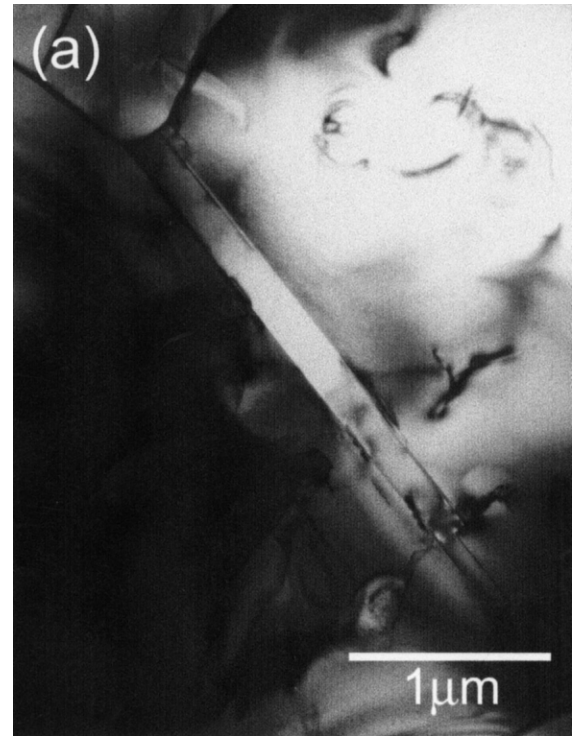
Fig. 2. TEM micrograph of \text{Ba}(\text{Mg}_{1/3}\text{Ta}_{2/3})\text{O}_3 materials incorporated with 0 mol% \text{Ba}_5\text{Ta}_4\text{O}_{15} , BaT, materials; showing a midrib running across the whole grains, which are of 8 layer periodicity.
