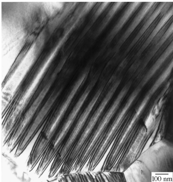
Fig. 4. Bright-field (BF) TEM image showing 90° domains in 2.4 mol% Nb-doped PZT (Zr:Ti ratio: 1.095).
