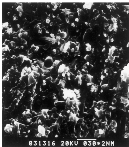
Fig. 5. Fracture surfaces after creep test under 500 MPa at 1100°C for 16 h.
