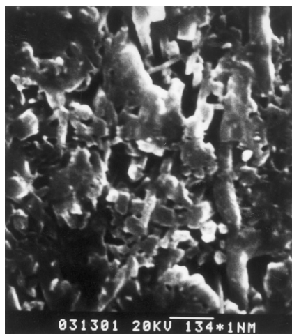
Fig. 4. The microstructure of Si 3 N 4 /BN fibrous monolith after creep under 350 MPa at 1200°C for 100 h.
