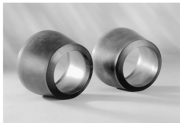
Fig. 3. Ceramic combustor exit cones of HIPed \text{Si}_3\text{N}_4 (CSN 101). The inner and outer surfaces are used with as-HIPed surface finish.
