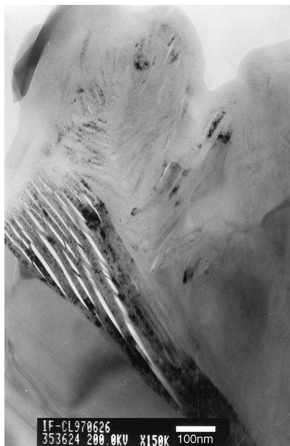
Fig. 2. TEM micrograph of textured, crystalline boron nitride formed near the original silicon nitride green body surface. The silicon nitride body has been facing encapsulation glass containing boron oxide during the HIP cycle. The apex of the wedge-shaped BN area points inwards. Adjacent grains now consist of silicon oxynitride.
