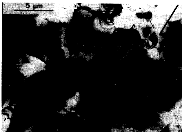
Fig. 1. Anisotropic cavity distribution in AlN after deformation by four-point bending (tension side) at T = 1873 \text{ K} , \sigma = 80 \text{ MPa} , \epsilon = 0.8 \times 10^{-2} . The stress axis is parallel to the marker.
