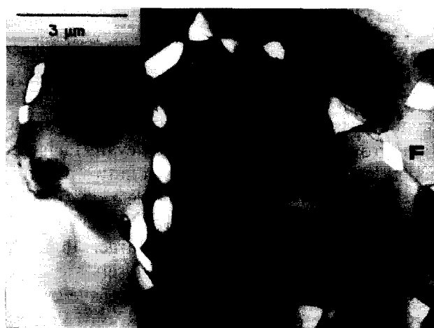
Fig. 4. Facetted cavities (F) in AlN after creep in compression ( T = 1873 \text{ K} , \sigma = 250 \text{ MPa} , \epsilon = 2.3 \times 10^{-2} ). Dislocations (D) and one inversion domain boundary (I) can be seen in one grain.
