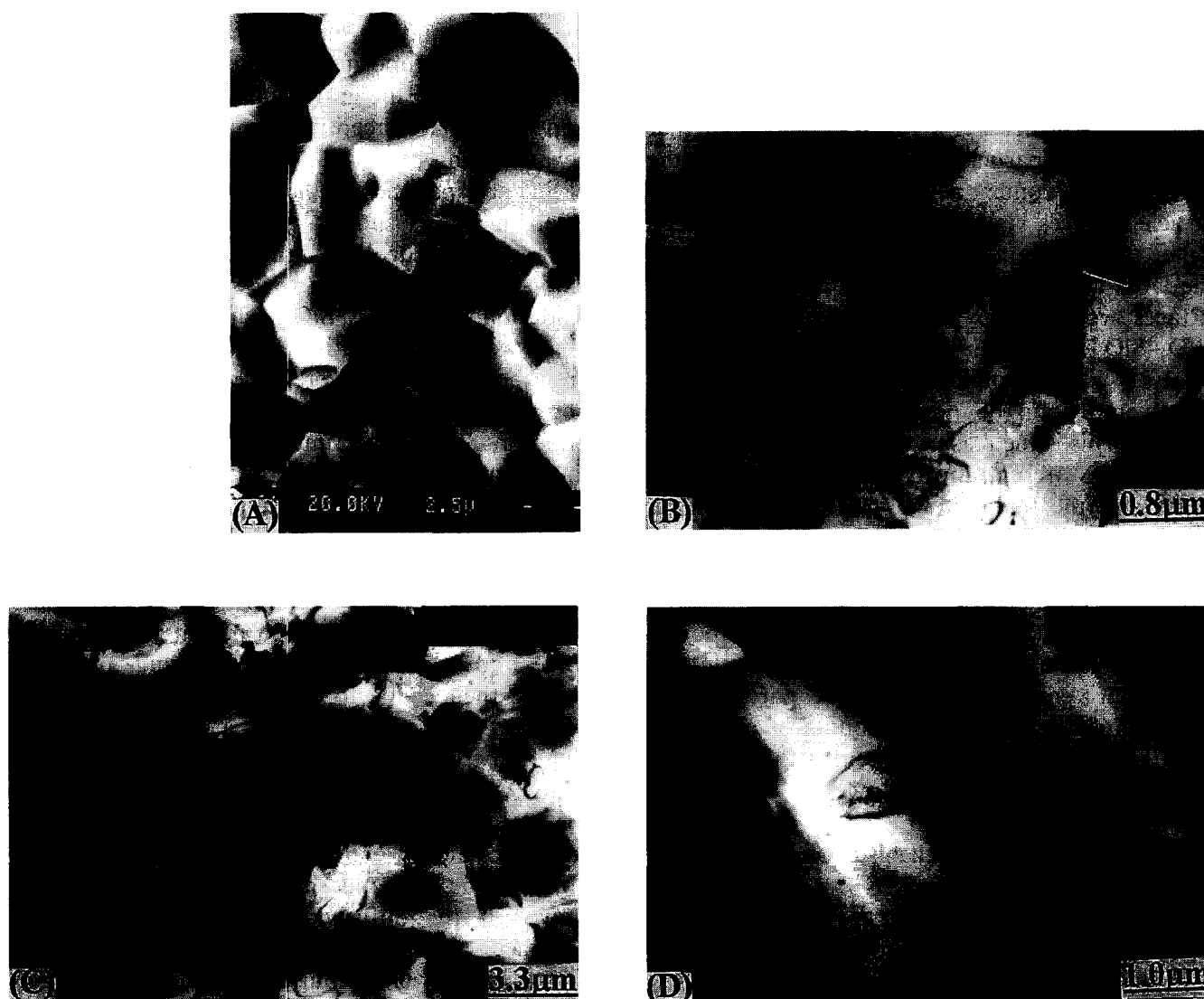
Fig. 4. Grain morphology of as-received specimens: (A) SEM micrograph of the fracture surfaces of monolithic \text{Al}_2\text{O}_3 ; (B) TEM micrograph of ASS; (C) and (D) TEM micrographs of ASL.
