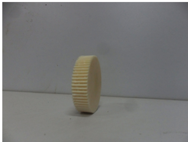
Fig. 13. Photograph of a near-net-alumina shape fabricated by the gelcasting process.
