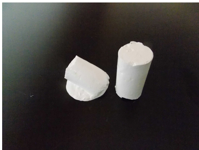
Fig. 6. Photograph of gelcast wet alumina bodies prepared at HMDA to formaldehyde mole ratio of 1 (left) and 1.1 immediately after mold removal.
