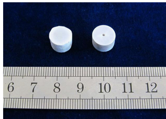
Fig. 1. Appearance of spark-plasma sintered precursor (left) and melt-grown eutectic rod (right) of \text{Al}_2\text{O}_3/\text{ZrO}_2/\text{YAG} ceramics.
