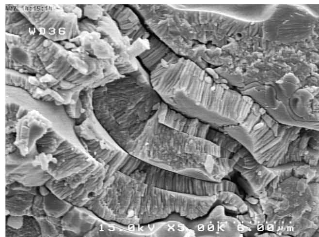
Fig. 2. FESEM micrograph of the fractured cross section of as-sprayed conventional YSZ coating.
