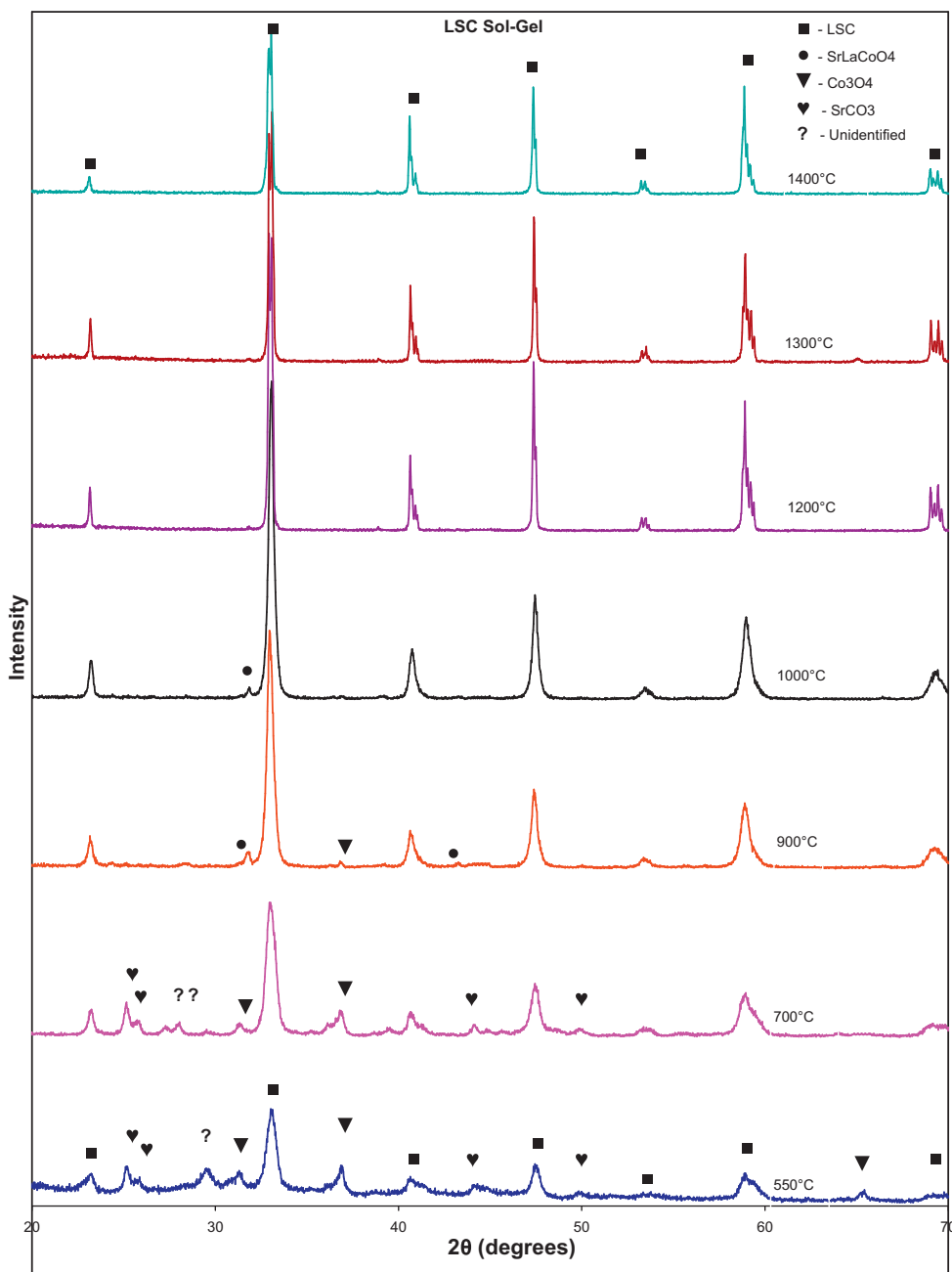
Fig. 3. X-ray diffraction patterns of \text{La}_{0.6}\text{Sr}_{0.4}\text{CoO}_{3-x} sol-gel nanopowders calcined at various temperatures.
