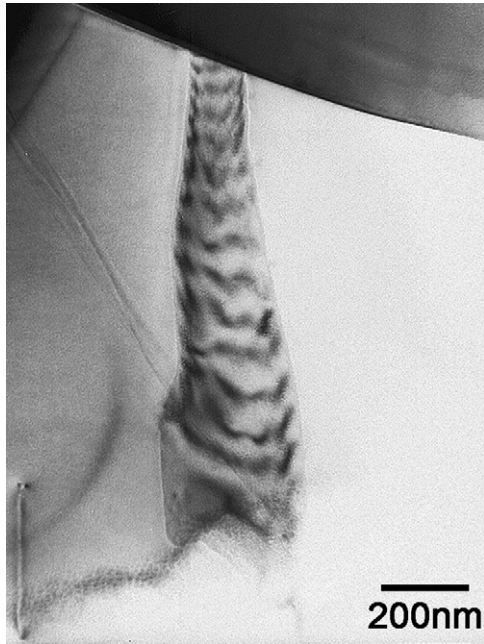
Fig. 3. TEM image of a 180° domain in a LiTaO 3 grain of the 15 vol.% Al 2 O 3 /LiTaO 3 composite ceramic.
