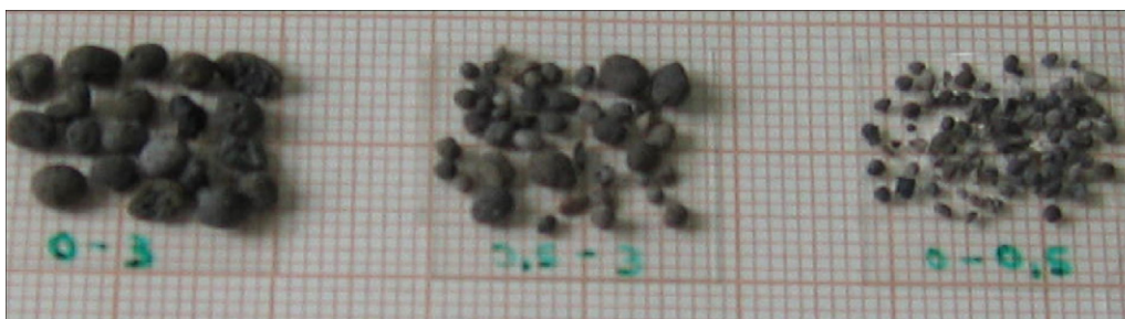
Fig. 2. View of lightweight clay aggregates sieved fractions (from left to right): 0/3 mm, 0.5/3 mm, 0/0.5 mm.
