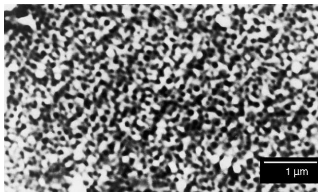
Fig. 4. SEM micrograph of specimen Z 2 after heating at 1073 K for 1 h, showing an interconnected microphase separation (bar = 1 μm).
