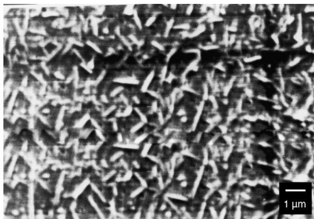
Fig. 8. SEM micrograph of specimen C 2 after heating at 1123 K for 1 h, showing crystalline particles of oxyapatite (bar = 1 μm).
