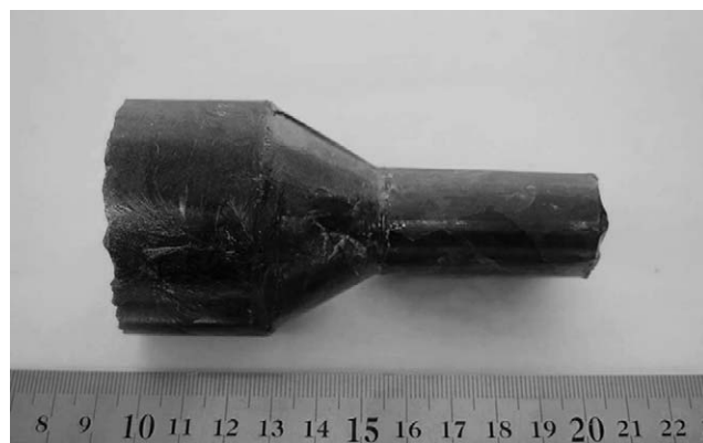
Fig. 2. PGO crystal grown by the vertical Bridgman method.
