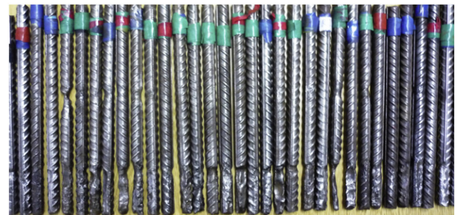
Fig. 5. Corroded reinforcement bars after cleaning.
