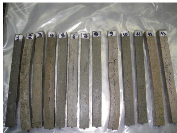
Fig. 12. Specimens stored, for one year, in the Na 2 SO 4 solution.
