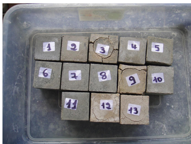
Fig. 11. Cubes stored, for one year, in the Na 2 SO 4 solution.
