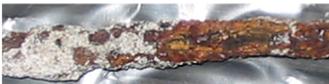
Fig. 2. Surface of top steel bar in one of the specimens exposed to \text{CaCl}_2 for 130 weeks.
