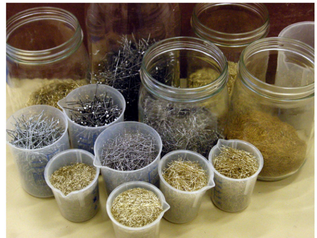
Fig. 2. Apparent volumes occupied by identical mass of fibers in random packing for various fibers aspect ratio.
