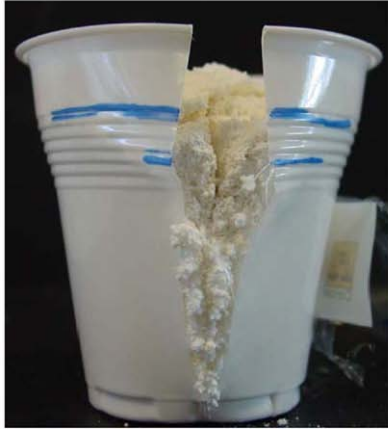
Fig. 1. Expansive gypsum plaster paste made with 20% calcium acetate solution. The lower horizontal line marked on the side of the cup represents the initial height of the fluid paste, and the upper line represents its final height (at the circumference). The cup is shown as found; the split in the side was solely due to the expansive reaction, and the apparent gash in the hardened paste appears to have been due to a combination of shear forces produced during partly-restrained expansion and drying shrinkage occurring afterwards, once the hoop constraint had been released due to the splitting of the cup.
