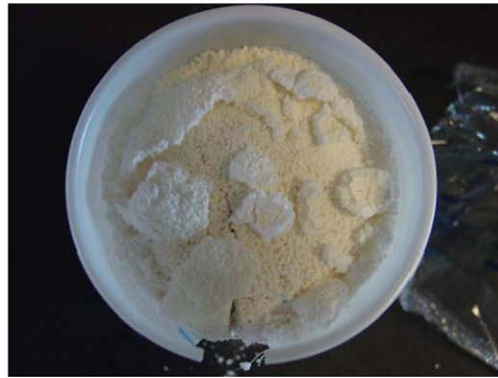
Fig. 1. Expansive gypsum plaster paste made with 20% calcium acetate solution. The lower horizontal line marked on the side of the cup represents the initial height of the fluid paste, and the upper line represents its final height (at the circumference). The cup is shown as found; the split in the side was solely due to the expansive reaction, and the apparent gash in the hardened paste appears to have been due to a combination of shear forces produced during partly-restrained expansion and drying shrinkage occurring afterwards, once the hoop constraint had been released due to the splitting of the cup.
