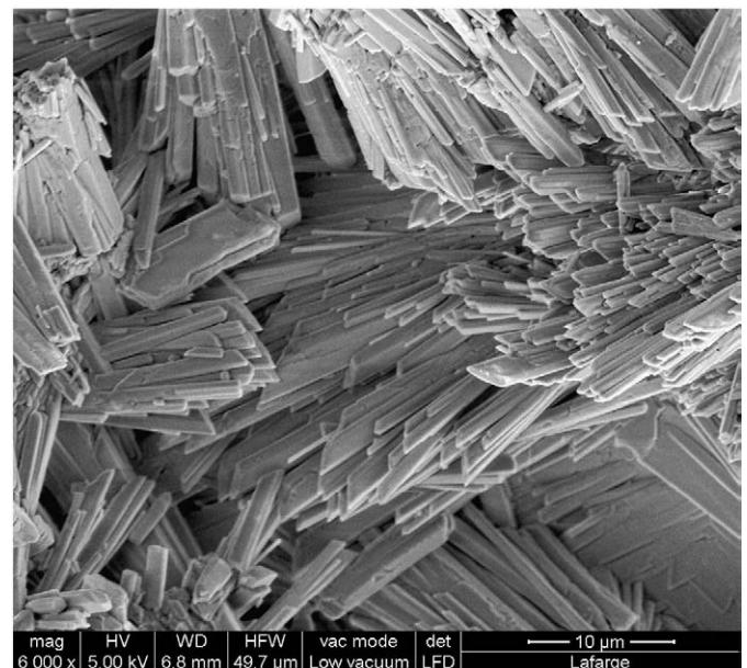
Fig. 2. Scanning electron micrograph of a fracture surface of a hardened plaster without admixtures.
