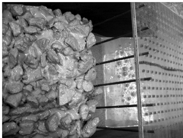
Fig. 5. Measurement method of the residue using an inclined channel. (Photo) test result for a SCC.
