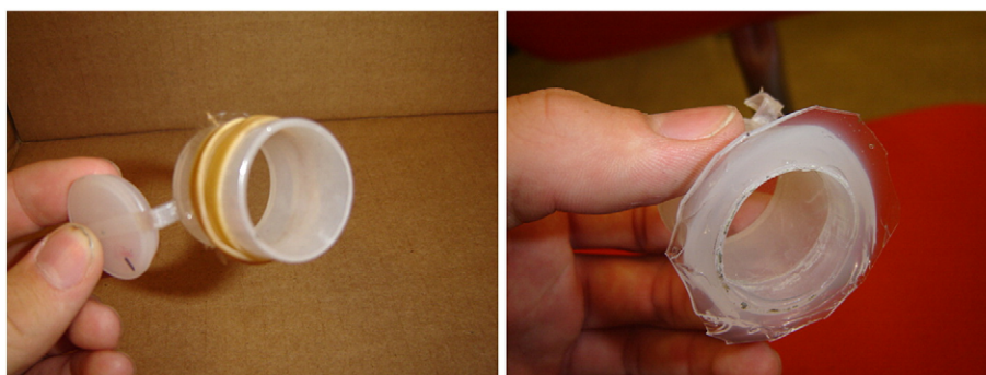
Fig. 2. Sample holders for acoustic emission measurements on fresh cement pastes. Left: sample Holder B with a flexible plastic film base (Saran wrap). Right: sample Holder C with an acetate sheet base (transparency) that is held in place with a bead of silicone.
