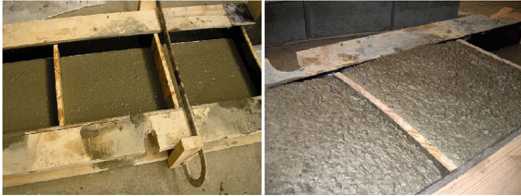
Fig. 7. Surface roughnesses for SCC N°1 (left) and SCC N°4 (right).
