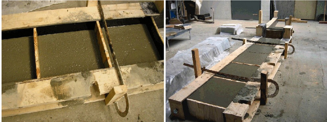
Fig. 4. Casting protocol. (left) After the first layer casting; (right) after the second layer casting.
