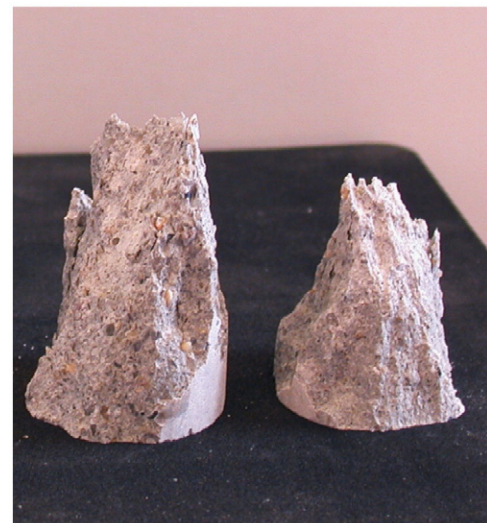
Fig. 11. Failure mode under uniaxial compression.
