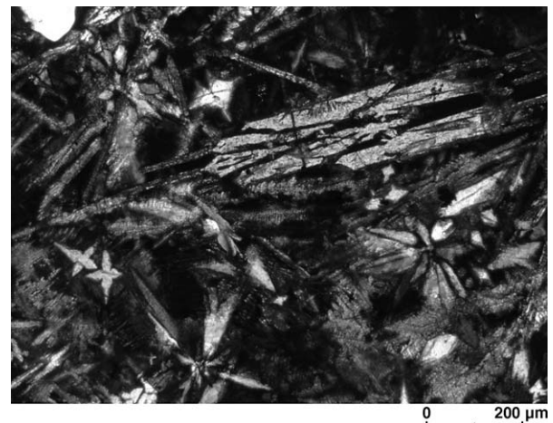
Fig. 4. Hedenbergite crystals in a MSWI bottom ash aggregate (photomicrograph, transmitted light, crossed Nichols).
