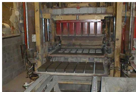
Fig. 3. Tray of paving blocks moving out of compaction machine in factory.
