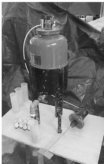
Fig. 2. The penetrability meter used in the experiments.
