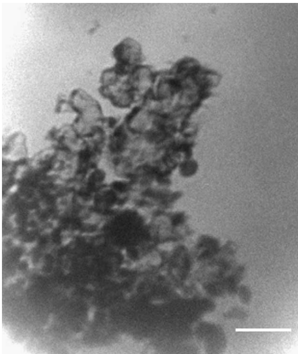
Fig. 6. X-ray image of \beta -( \text{Ca}_{1.84} + \text{Ba}_{0.16} ) \text{SiO}_4 prepared with hydrothermal treatment of 150 °C in water after 20 min; the image was taken with an exposure time of 12.753 s and a beam current of 233.8 mA.
