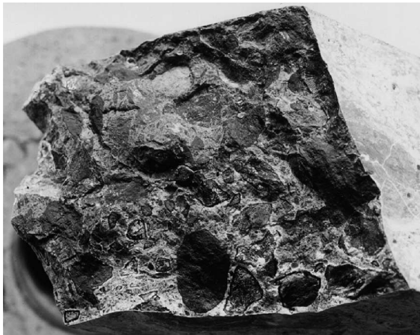
Fig. 4. Break surface of a concrete prism, showing white gel and classic dark reaction rim around some aggregates.
