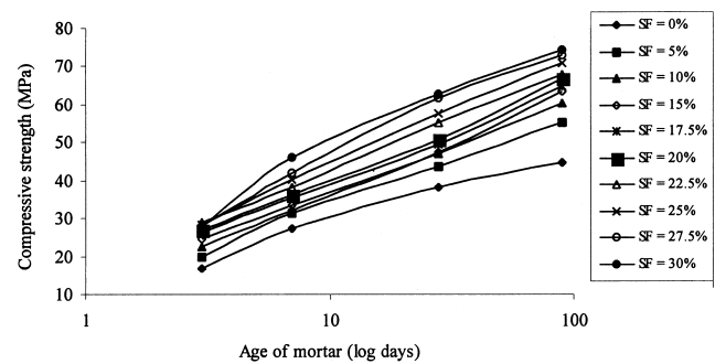
Fig. 4. Variation of compressive strength of mortar with age (log scale) at different silica fume contents at w/b ratio of 0.50.
