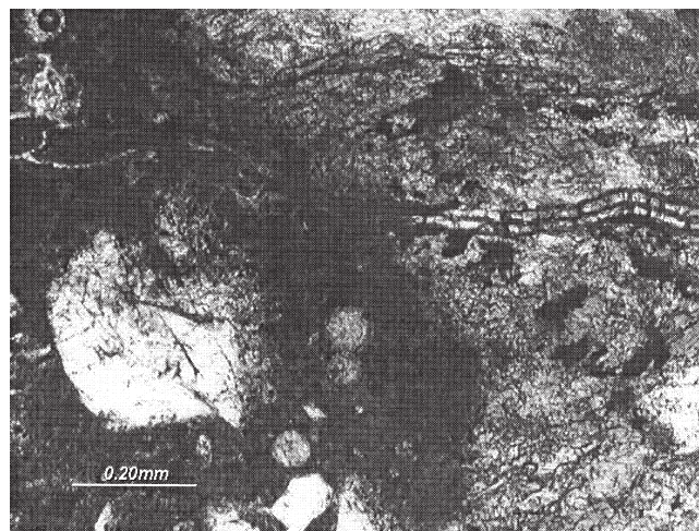
Fig. 3. Thin section of pavement shown in Fig. 1. The crack in Hylas particle is filled with reaction product and extends through the paste.
