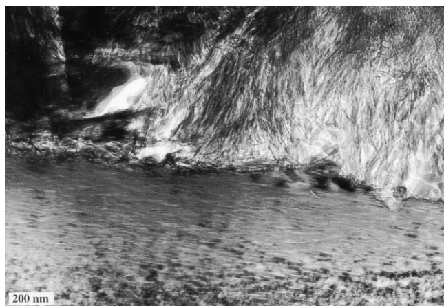
Fig. 7. Transmission electron micrograph showing fine fibrillar Op C-S-H (top) and CH in a mature Portland cement paste.
