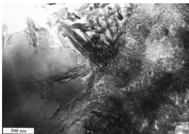
Fig. 25. Transmission electron micrograph showing fibrillar Op C-S-H well-bonded with CH in a C 3 S paste hydrated for 3 1/2 years at 20°C (W/C = 0.4).
