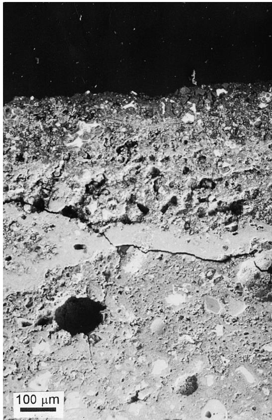
Fig. 3. Backscattered electron image of a cut cross-section of the leached surface (top) after 210 days.
