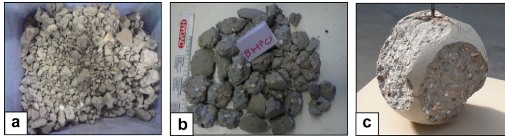
Fig. 12. Samples after spalling for a sphere diameter of (a) 0.12 m, (b) 0.18 m and (c) 0.24 m – No fibre concrete mixtures (HPC0).
