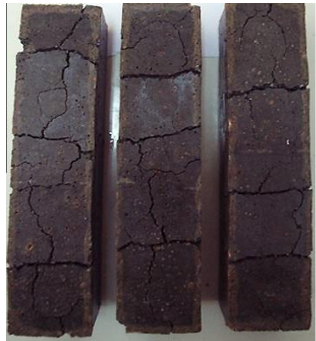
Fig. 5. Plain Portland cement (A) prismatic mortars exposed to sodium sulphate solution for 36 months.
