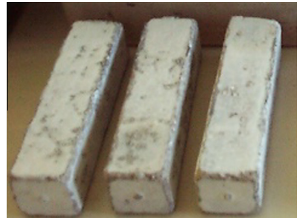
Fig. 4. Selected blended cement prismatic mortars (C 2 ) exposed to sodium sulphate solution for 36 months.
