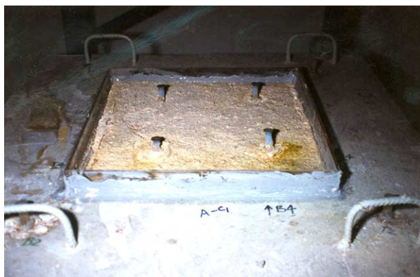
Fig. 10. Control concrete specimens exposed to sulfuric acid.
