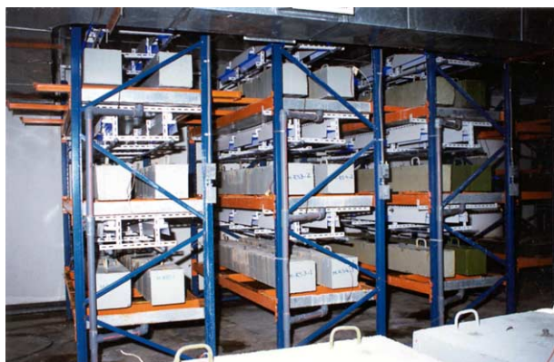
Fig. 6. Concrete beam specimens exposed to salt spray and UV light (marine exposure).
