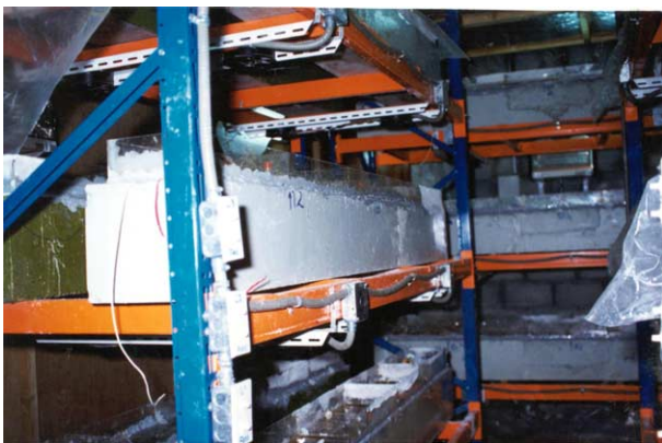
Fig. 9. Control and repaired concrete beam specimens exposed to belowground conditions.
