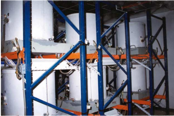
Fig. 8. Repaired and control slab specimens exposed to potable and saline water.
