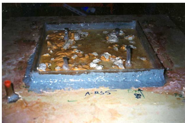
Fig. 11. Concrete specimens repaired with system 5 and exposed to sulfuric acid.
