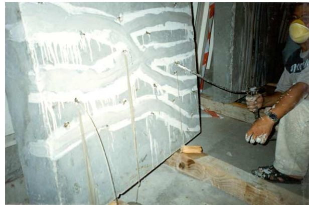
Fig. 5. Repair of cracks in the slab specimens by epoxy injection.
