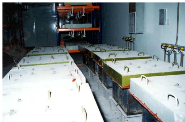
Fig. 7. Concrete slab specimens exposed to sulfur fumes.
