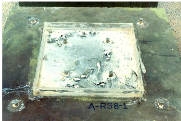
Fig. 12. Concrete specimens repaired with system 8 and exposed to sulfuric acid.
