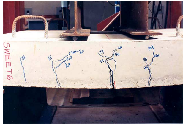
Fig. 4. Close-up view of a cracked concrete specimen.
