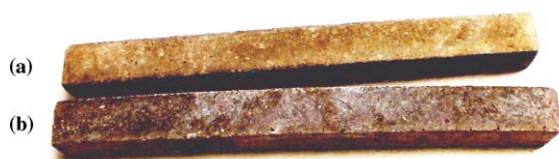
Fig. 2. Mortar specimens with hydrophilic siloxane admixture. (a) After 48 h of autoclave testing. (b) After ASTM C1260 testing (note in Figs. 2 and 3: different color, visibly larger expansion, bar distortions, and surface cracking after ASTM C1260 testing).
