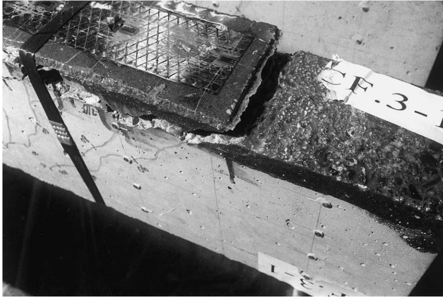
Fig. 17. Major shear crack at the end of epoxy mortar layer.
